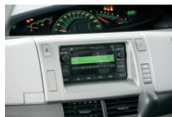
The audio system features AM/FM radio and a single disc in-dash MP3/WMA CD player. Sound can be controlled from the dash or by the driver from steering wheel controls.
